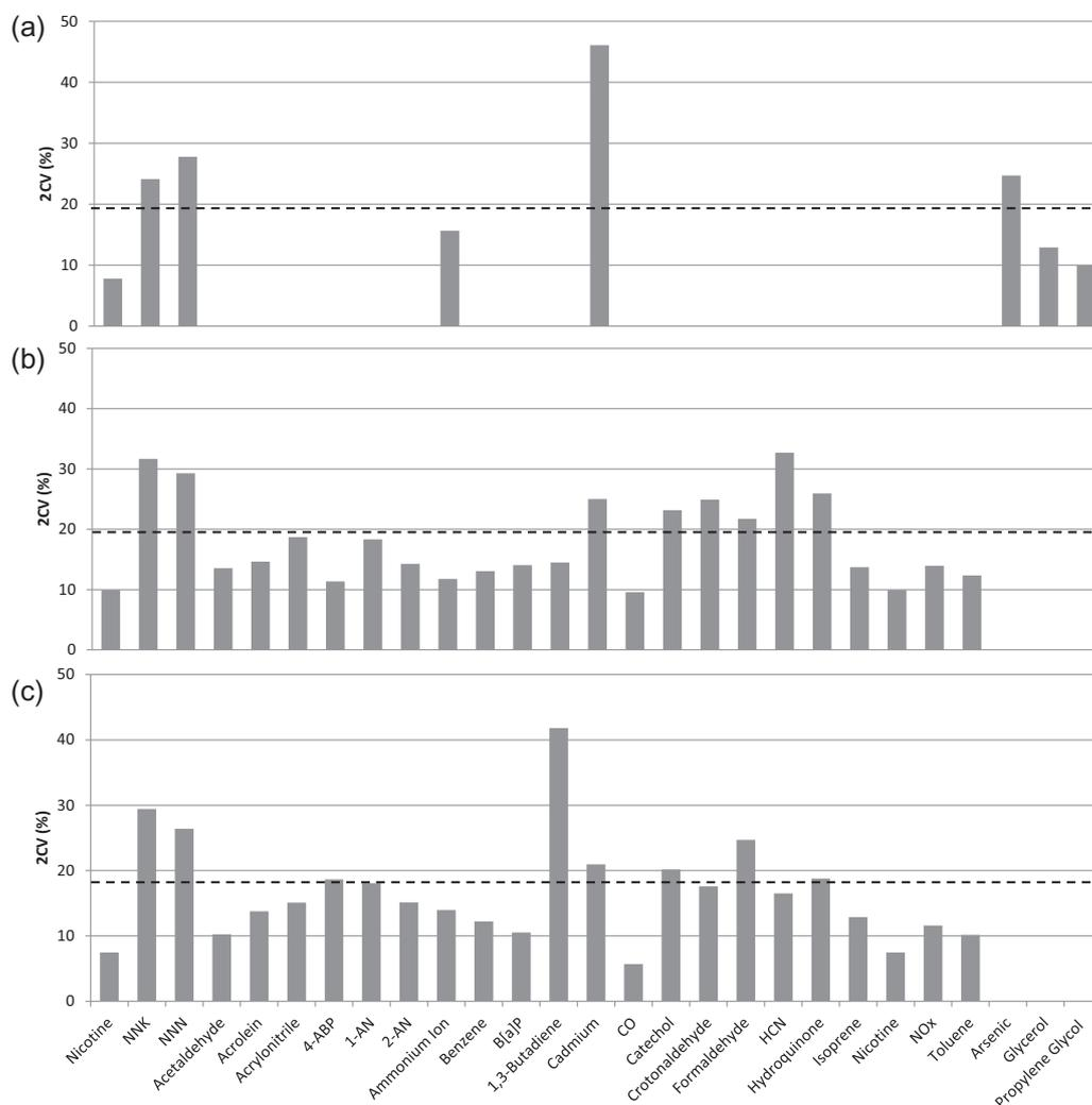
**Fig. 5.** Potential error associated with single-point-in-time analysis of toxicants of regulatory interest for commercial, high-volume cigarette products: (a) filler blend components, (b) toxicant emissions under ISO regime, (c) toxicant emissions under HCl regime. The dotted black line shows the median value for each of the 3 categories.
